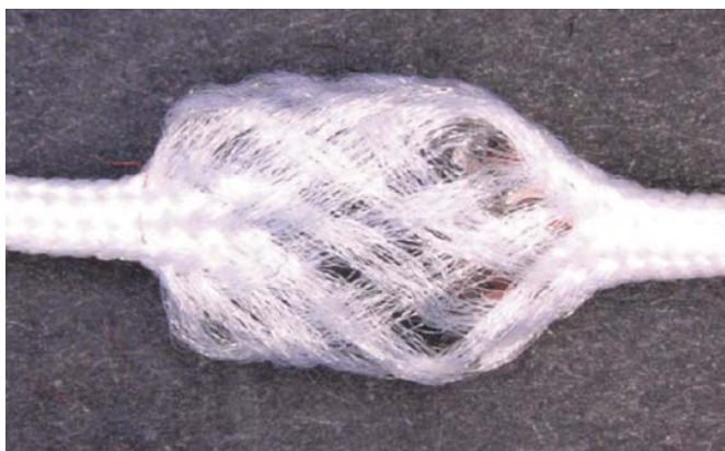
The smart over-sock, which features a tiny motion sensor embedded in yarn, embedded at the ankle, can be connected to an internet-enabled device, such as a smartphone, via a detachable microcontroller using Bluetooth. Photo: Nottingham Trent University
