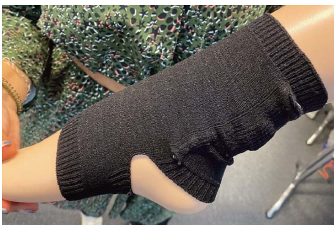
A smart over-sock has been designed at Nottingham Trent University with an embedded inertial motion unit to detect fall events for older adults. It can differentiate between “activities of daily living” (ADLs) and falls with an accuracy of 99.4%, and between ADLs, falls and stumbles (near-falls) with an accuracy of 94.2%. Photo: Nottingham Trent University
