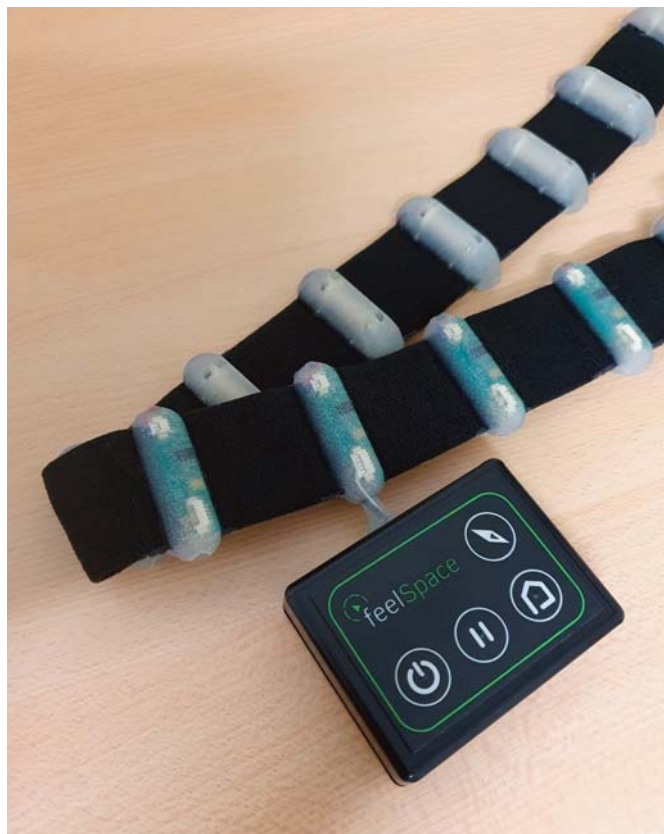
Demonstrator manufactured using ultrasonic welding. Photo: FeelSpace
