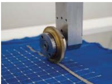
Roll-to-roll thermoplastic ultrasonic welding conductive ribbons on embroidered testing pattern. Photo: University of West Bohemia
